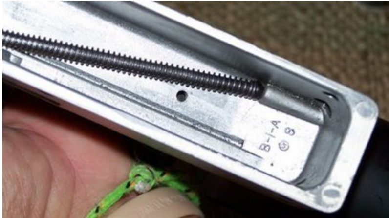
Install guide rod and charging handle.
