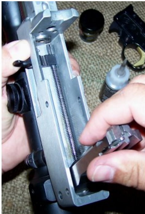
Insert bolt in rear of action
