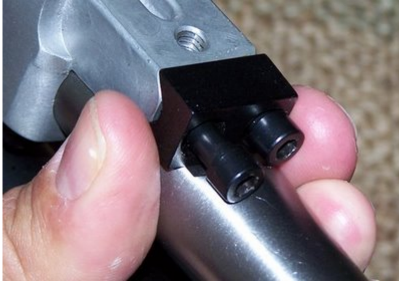
Install V block screws.
