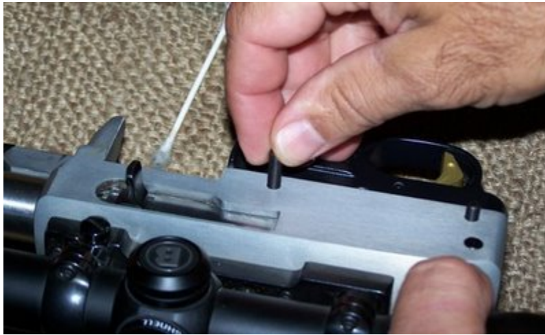
Insert trigger group pins.
