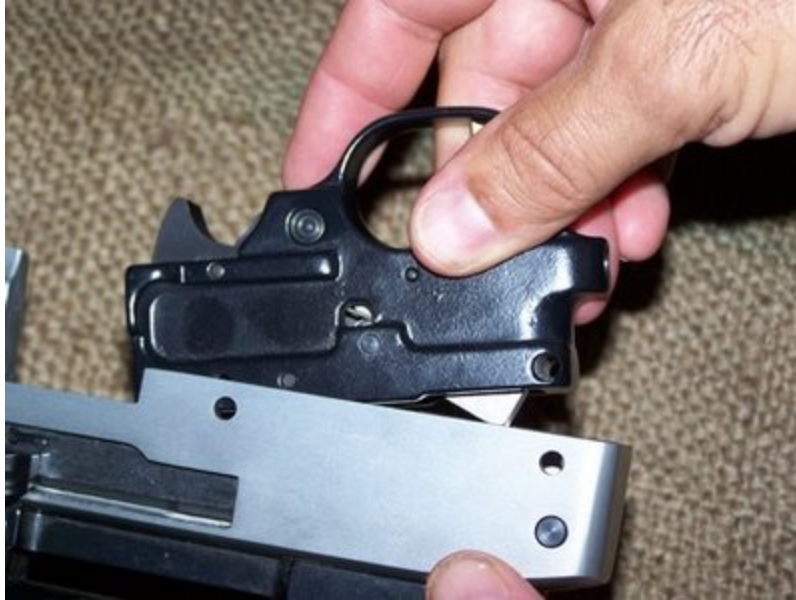
Insert trigger group with hammer back.
