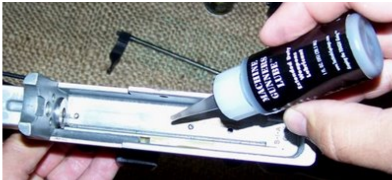
Lubricate action sparingly.
