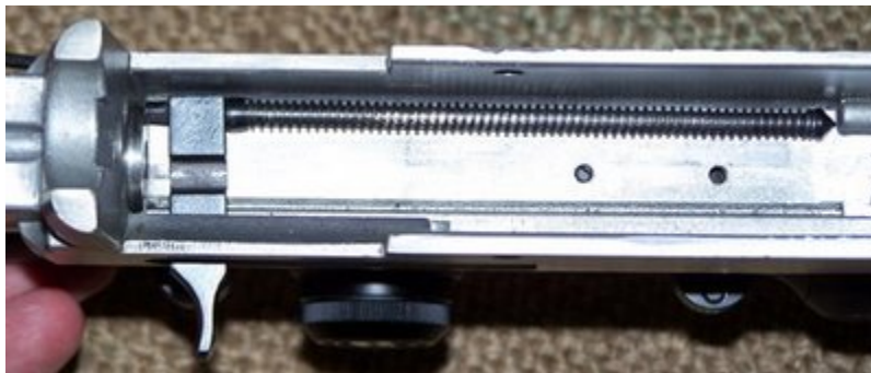
Guide rod and charging handle in place.
