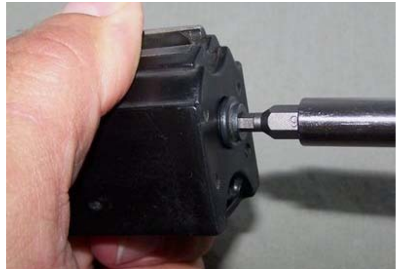
Now, gently tighten the screw making sure it threads properly. You do not need to wrench it down like a lug nut!
