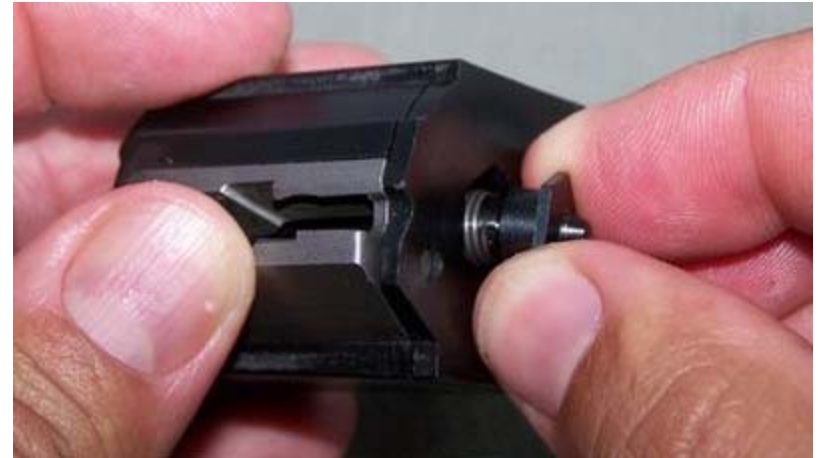
Rotate the end cap nut eight notches (flats on the hex) clockwise, and press it in place. I found it easiest with my fingers holding the nut and the other hand rotating the magazine. Then I used my thumb to help press the nut in place.
