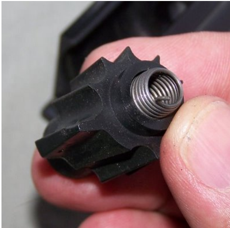
Note the little tab on the end of the spring, and the long vane on the rotor.
