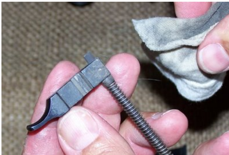
Don't forget to clean the spring and guide rod too.
