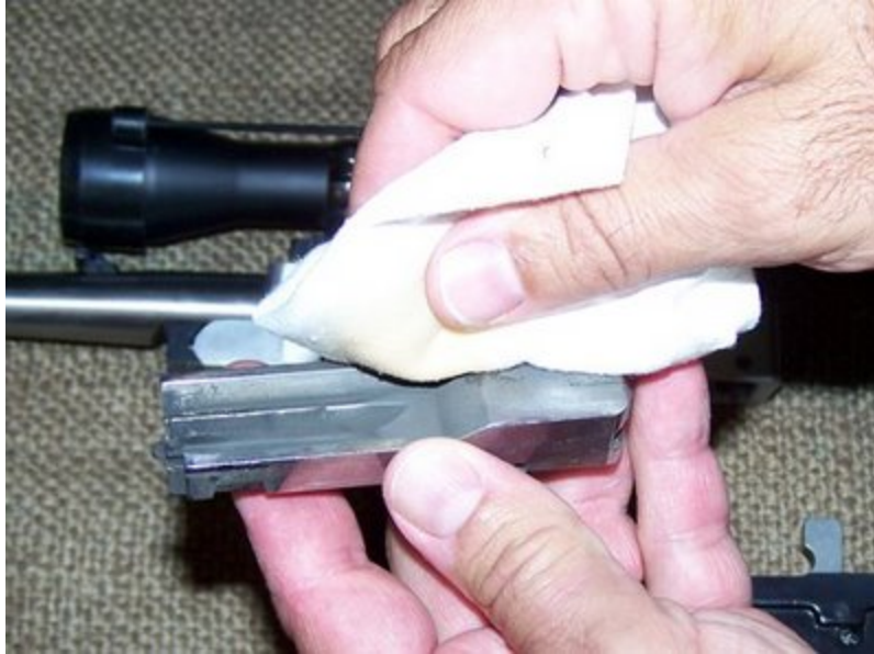
Scrubbing the bolt clean.
